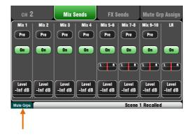
**Function Key** – The **Fn** key provides access to further options associated with the currently selected screen, for example channel source selection and processing libraries. If available, its function will appear in the lower toolbar above the key. Press the key again to close the option screen.
