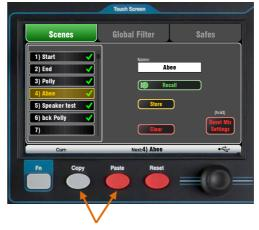
**To Copy a Scene** – Press and hold the Copy key below the screen and then touch the scene to copy. Now press and hold the Paste key and touch the scene in the list to paste to. This copies the scene contents and name.
