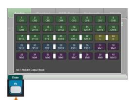
This screen presents the patching of the dSNAKE remote audio outputs. These outputs have a fixed mapping as shown here. This suits the typical application.
