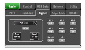
Set up and assign the Signal Generator to test loudspeakers and align levels between equipment.
