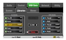
Individual processing Libraries can be transferred between Qu mixers via a USB device (key or drive) plugged into the Qu-Drive port. Make sure the USB device has been previously formatted using the Qu mixer Utility / Qu-Drive screen.
