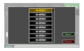
**Qu-Drive Multitrack page** – This screen presents the controls for multitrack recording to and playback from a USB hard drive plugged the top panel Qu-Drive port.
