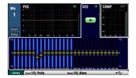
Press the **GEQ Fader Flip** key to view and adjust the GEQ on the faders while a mono or the LR mix is selected. The screen highlights the active range of frequencies. Press the switch again to change range or return to normal mix mode.
