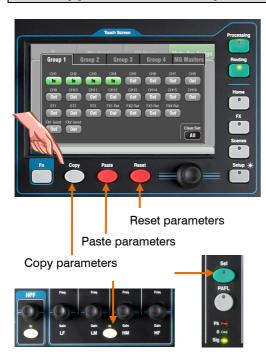
Press + hold down one of these keys and then press another key or screen item to copy, paste or reset the related parameters. For example:
