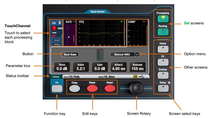
**Button** – Touch to select its function or change its state. To avoid accidental operation some functions need be touched for at least 1 second, for example switching 48V phantom power. These are marked '(Hold)'.
