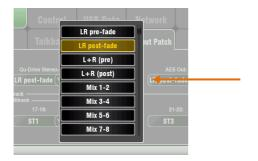
Patch the source to be recorded using the Setup / Audio / Output Patch screen Qu-Drive option menu. The record meter on the USB page displays the current source. The default is LR post-fade.
