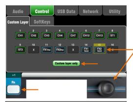
The following strip types are available: Х Unassigned CH Mono input channels 1-16 ST Stereo input channels 1-3 **FX** Ret FX returns 1-4 FX Send FX sends 1-2 Mix Mix masters 1-10 LR Main LR master MIDI MIDI DAW control
