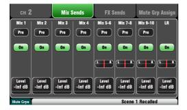
**Routing Screen** – When selected this screen lets you access the assignment and routing for the channel or master currently selected using its strip **Sel** key.
