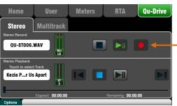
**Stereo Record** – You can record to a USB hard drive plugged into Qu-Drive:
