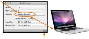
Two squares in the status bar flash to display MIDI I/O activity. To check you are connected to the mixer, the left square should flash when you move any Qu fader.
