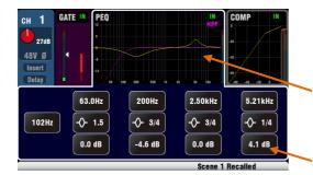
**Processing Screen** – When selected this screen presents the processing such as Preamp, EQ, Gate, Compressor for the channel or master currently selected using its strip **Sel** key.
