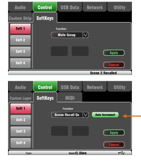
Qu-16 features 4 SoftKeys. These are called 'Soft' because they can be assigned to different functions by the user.
