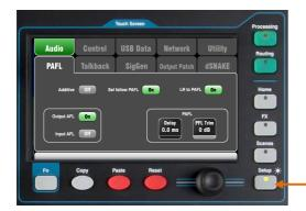
Touch the top tabs to access the different categories of setup function. Touch the tabs below to open up the related options available.
