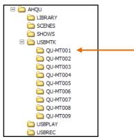
Note – We recommend you transfer previous recordings to your computer and then reformat the USB drive on the Qu mixer before using it for each show. This will avoid potential audio skipping that may occur with some hard drives containing long recordings.
